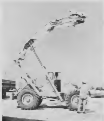
The 4-ton Pettibone Super 8 High-Lift can lift up to 18 feet through hydraulic gear.
